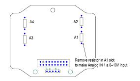
Step 1. Cut out the resistor installed in the A1 (analog 1) slot. (Your wiring board may differ slightly from the board shown. Use the board's labels to confirm you have selected the correct resistor to cut.)
